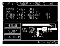
▲ Figure 2.7(b) Measurement Screen (Battery Operation)
