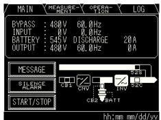
Figure 2.8 Main Screen (Fault Indication)
