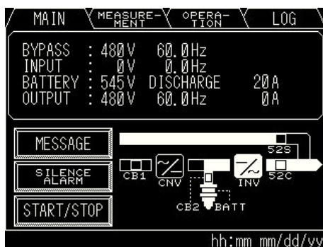
Figure 2.8 Main Screen (Fault Indication)
