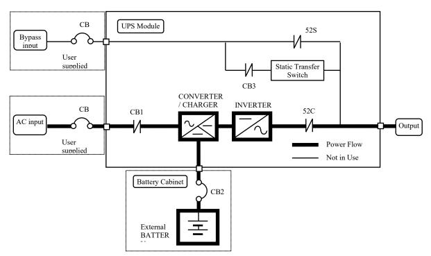
During normal operation, the path through the UPS inverter is used to power the load.
