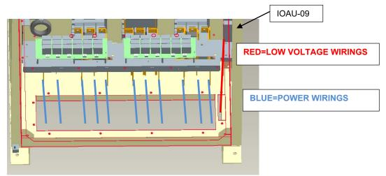
Figure 3.5 Cable Entry on Top (Example of 225kVA)
