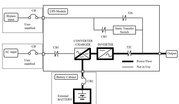
Figure 1.3 Single Line Diagram - Battery Operation
