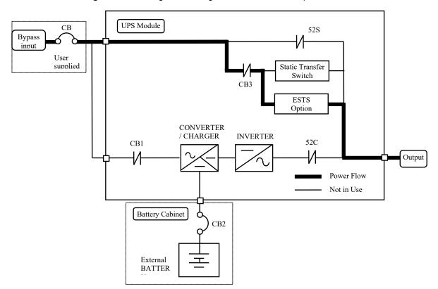
Figure 1.4 Single Line Diagram – Enviro-mode Operation
