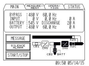
▲ Figure 2.7b Measurement Screen (Battery Operation)
