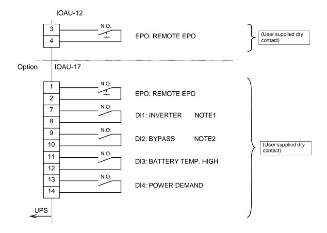
NOTE1: Remote transfer operation from BYPASS to INVERTER.
