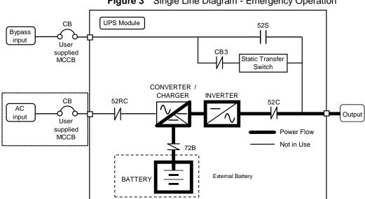
Figure 3 Single Line Diagram - Emergency Operation
