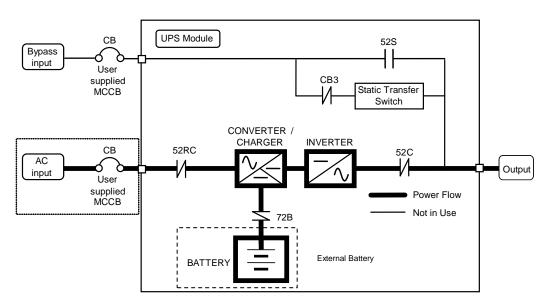
During normal operation, the path through the UPS inverter is used to power the load.
