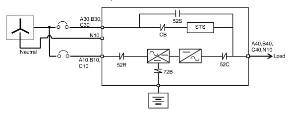
Figure 38 Cable Connection for Single Input
