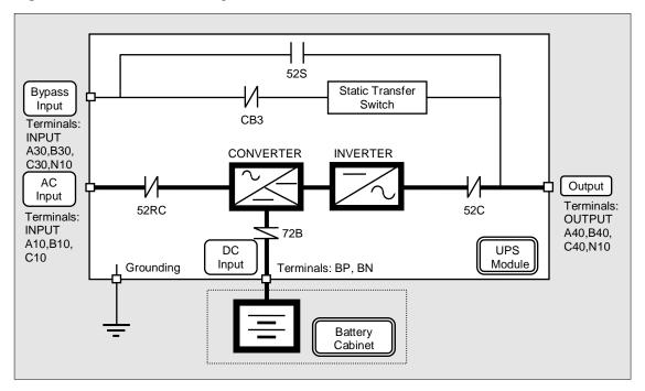
Figure 37 Cable Connection for Dual Input
