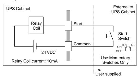
Details of input contacts for remote access: IOAU-12
